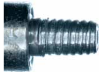
DAMAGED → Generic ultrasonic instruments overload the sonotrode and severely shorten its life span
