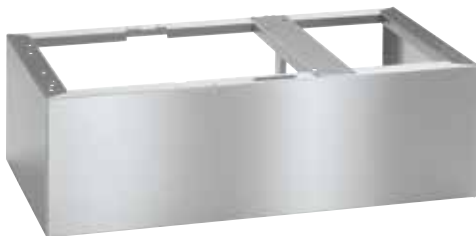
UG 30-90/60-85 plinth • For use with PG 8581 and PG 8591 in combination with PG 8596 dispenser housing unit • Stainless-steel plinth, bolted to machine • H 300, W 900, D 600 mm
