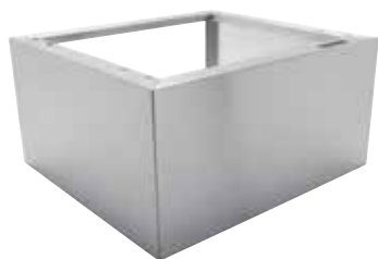
UG 30-60/60-85 plinth • For use on PG 8581 and PG 8591 • Stainless-steel plinth, bolted to machine • H 300, W 600, D 600 mm
